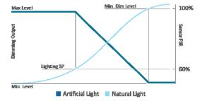
The daylight harvesting application can override the Auto-ON feature of occupancy sensors if the light level is sufficient and calls for the lights to be off.
